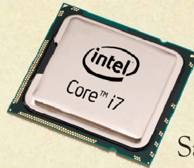
Ivy bridge de Intel (3D transistors)
