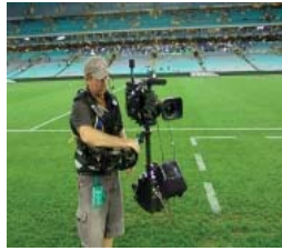
RF Camera installed on a steadicam
