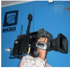
RF Camera carried to the shoulder
