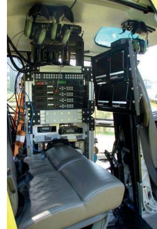
RF Mobile System installed in a relay helicopter
