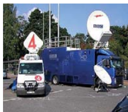
Satellite Van equipped with up-link antenna
