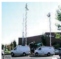
News van equipped with point to point RF Contribution System
