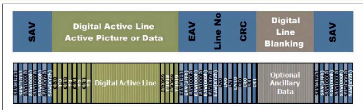
Figure 34. SDI data structure for a single line.
