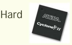
DES sequential on FPGA Cyclone II EP2C35 (~ 80 CHF)
